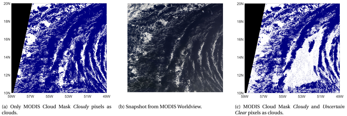
Figure 3.16: Differences in cloud classification on February 2, 2015 (TERRA) when only using MODIS Cloud Mask Cloudy pixels as clouds (a) or also considering MODIS Cloud Mask Uncertain Clear as clouds (c). A snapshot from MODIS Worldview (b) is added to compare.
