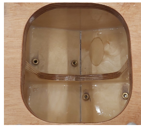
Figure 3.7: Inside construction of the wedge with 30° deadrise angle.
