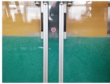
Figure 3.44: Snapshot of the moment just after impact. The spray can be seen. Also the flow can be seen compressed around the flat plate.
