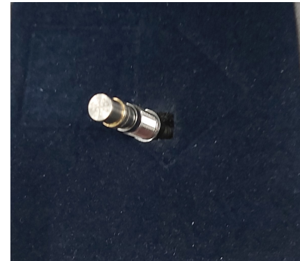
Figure 3.12: Piezoelectric PCB Pressure sensor including the clamp nut and seal ring used to install the sensors in the wedges.
