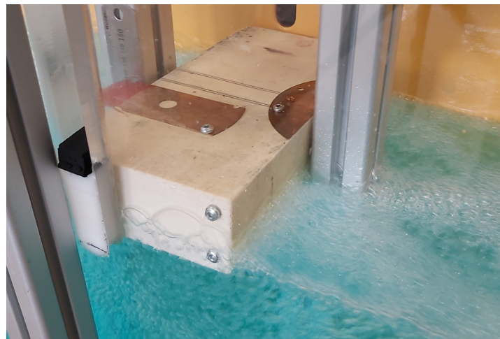
Figure 3.17: Float installed in the water. In order to clearly read the scale on the right side of the float, which can be seen in the picture behind the red indicator, the float must be restricted in its movement. If it is not confined, the float will move due to the circulation of the water. The movement is limited by the wooden back panel and the Plexiglas front panel as well as two Item profiles on the side. To allow upward and downward movement and to limit rotation, screws are attached to the foam block to guide it.
