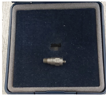
Figure 3.9: PCB piezoelectric Accelerometer installed in the upper block. The accelerometer is screwed into a plate fixed in the block.
