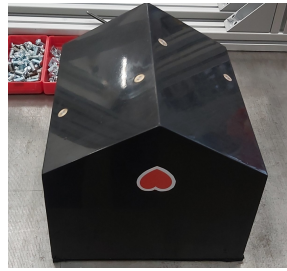
Figure 3.4: Wedge 30 with sensor locations, the installed sensors can be seen on both side of the wedge.
