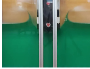
Figure 3.38: Snapshot of the Wedge with a deadrise angle of 15^\circ . After impact the flow forms towards a more typical flat plate impact.
