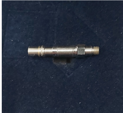
Figure 3.11: Piezoelectric PCB pressure sensor including the clamp nut and seal ring used to install the sensors in the wedges.
