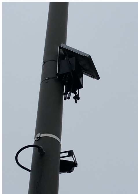
(a) Air quality sensor (top, with solar panel) together with a motion sensor (below) mounted on a lamp post
