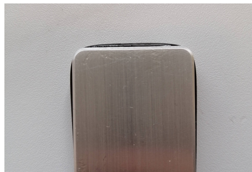
Figure 18. Side-view of a small O-ring (black) wrapped around the vane (silver). It is noticed that the O-ring is not visible at the roundings, indicating the O-ring is too thin at these locations.
