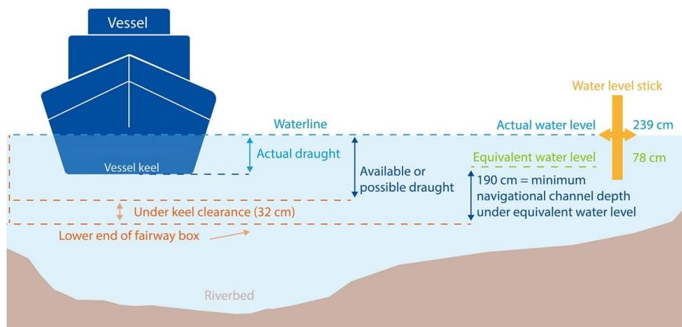
Figure 2.6: Explanation water level, equivalent water level, navigational channel depth and under keel clearance at Kaub (CCNR, 2021)
