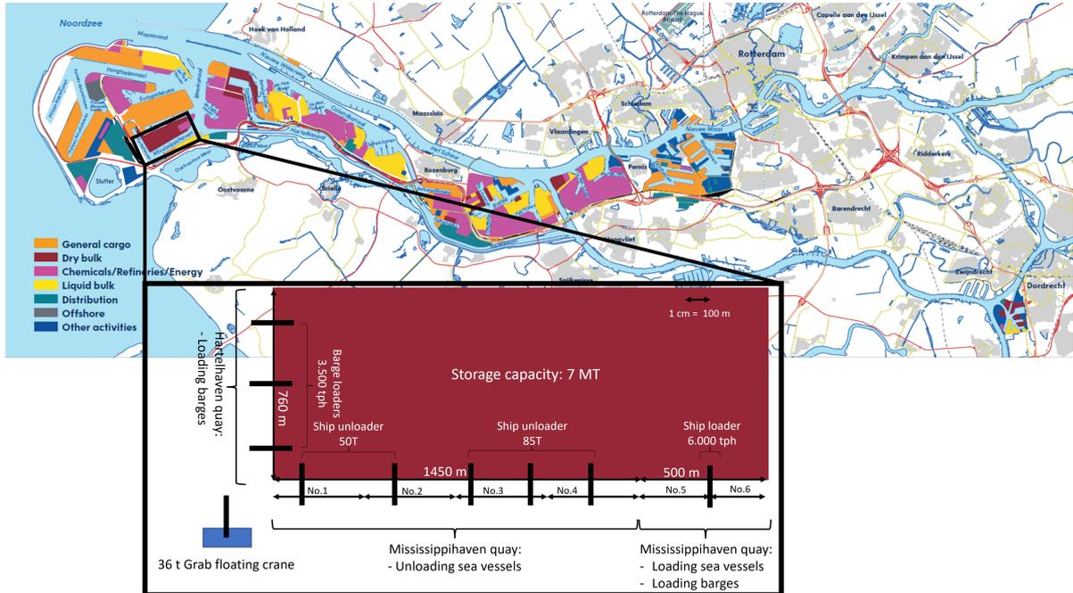
Figure 3.2: Map of Port of Rotterdam terminals with detailed EMO terminal layout (Port of Rotterdam, 2021)
