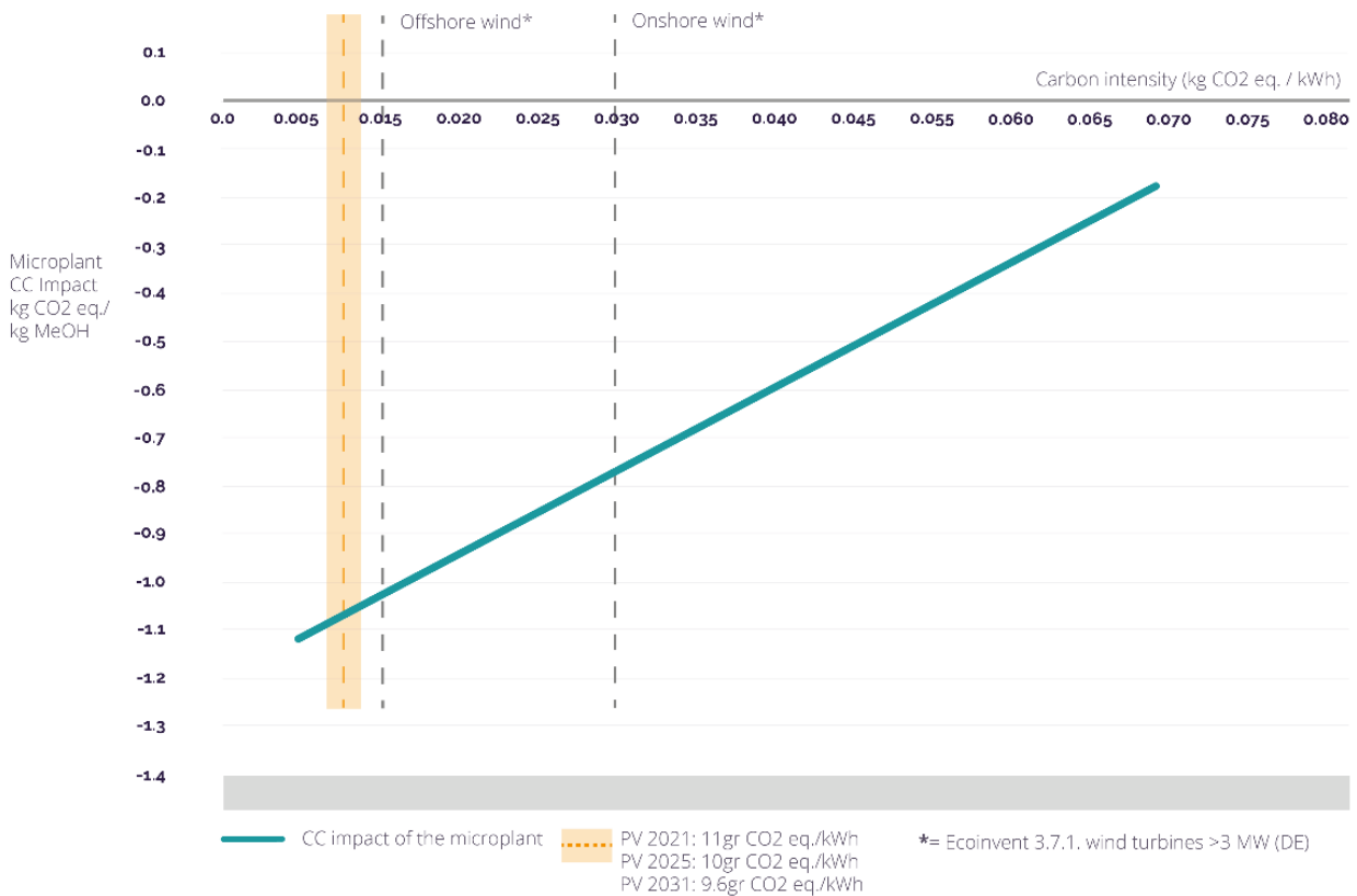
Figure 17: Climate Change impact score of the methanol produced by the microplant as function of the carbon intensity of the electricity supply
