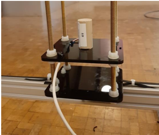
Fig. 3. The cart moving over the measurement rail. A magnetometer is placed on top of the cart, of which the height can be varied.
