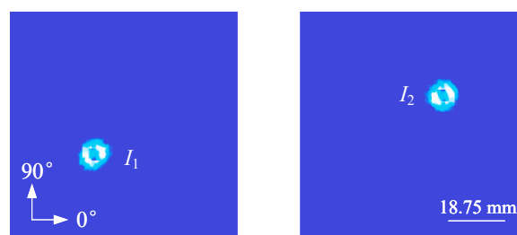
Fig. 11. Projected delamination areas of the single steel impact with the velocity of 22 m/s at impact locations of I_1 and I_2 , the delamination area of these two cases is 96.54 mm 2 .
