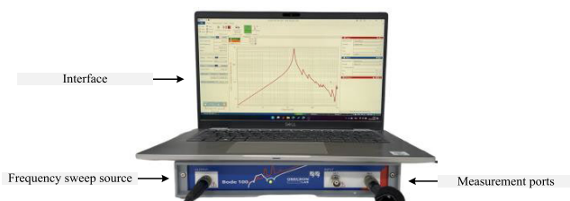
FIGURE 15. Example of transformer measurement using bode 100 VNA.
