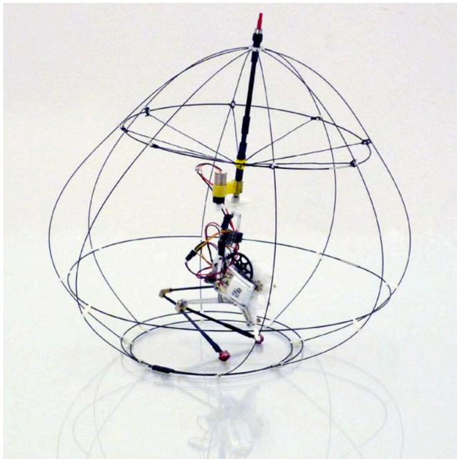
Figure 12: Picture of EPFL jumping robot [4], with lifting mechanism. The cage around the robot lifts the robot off the ground.
