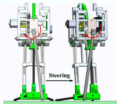
Figure 13: Robot by J. Zhang et al. [41] with lifting arm. The arm is visible in grey and the red arrow indicates the direction of rotation of the arm. On the left, the robot is in an unturned position. On the right, the arm has made a full rotation and the robot is rotated a bit.
