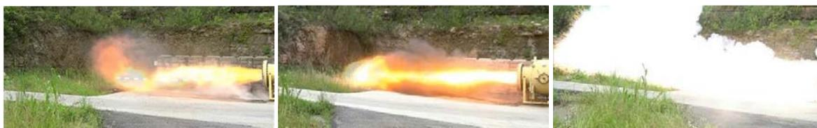
Figure 1: Photographs of 2-m<sup>3</sup> vented tests with cornstarch, iron and aluminium dusts (Taveau et al, 2019b)
