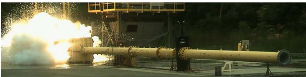
Figure 4: Mechanical explosion isolation of an aluminium dust ( $K_{St} = 450 \text{ bar m/s}$ ) deflagration initiated in a  $5\text{-m}^3$  vented vessel (Taveau, 2017)
