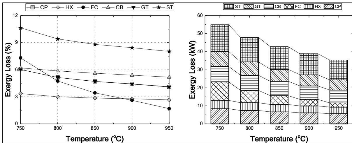
Figure 9. Exergy Loss variation v/s Cell Temperature - Hydrogen
