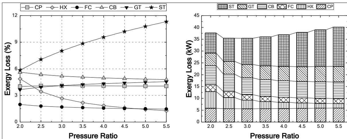
Figure 12. Exergy loss variation v/s Pressure Ratio - Hydrogen
