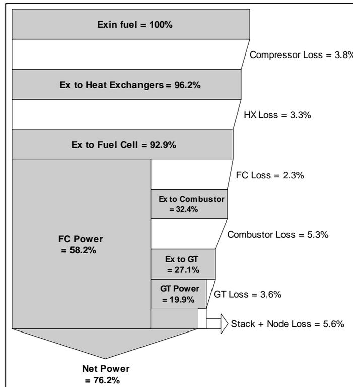
Figure 26. Exergy flow diagram – Hydrogen Optimized
