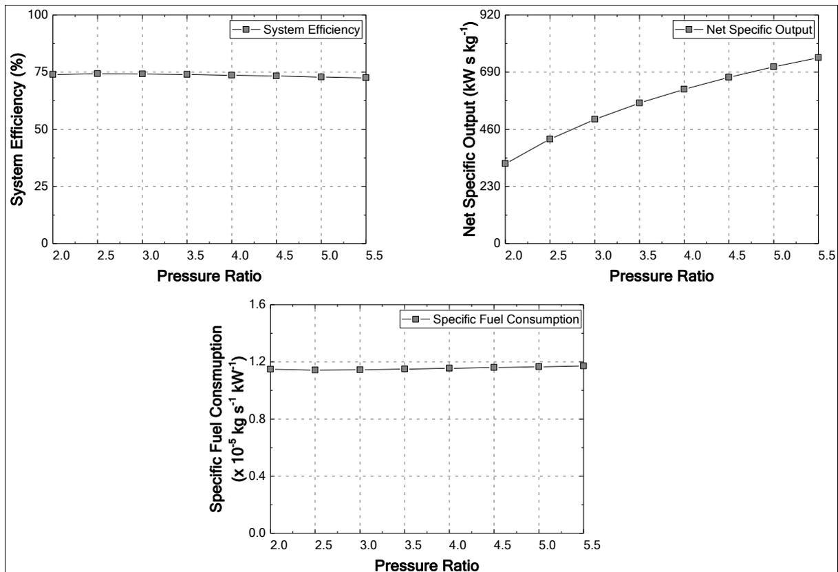
Figure 13. System Efficiency, Net Specific Output, Specific Fuel Consumption v/s Pressure Ratio - Hydrogen
