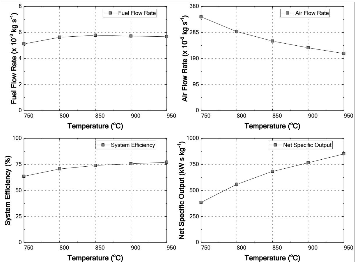
Figure 16. Trends in System Variables v/s Cell Temperature – Methane
