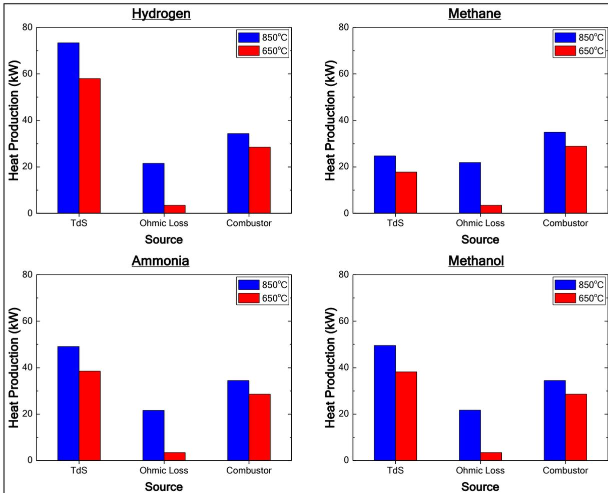
Figure 29. Heat Production distributions for all fuels at different temperatures
