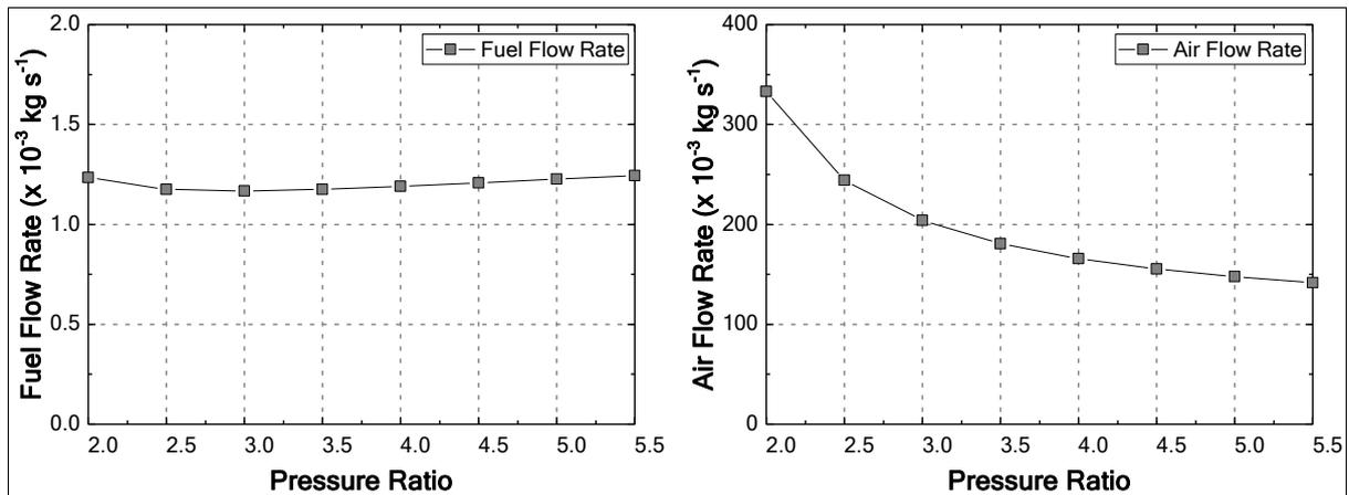
Figure 11. Fuel Flow, Air Flow v/s Pressure Ratio – Hydrogen
