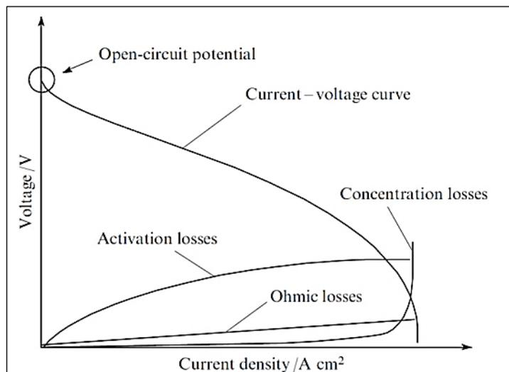
Figure 3. I-V curve of an SOFC with various losses [45]
