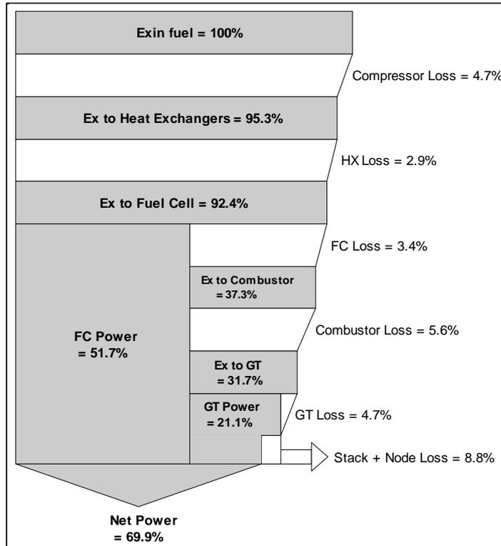
Figure 7. Exergy flow diagram – Base Case Hydrogen
