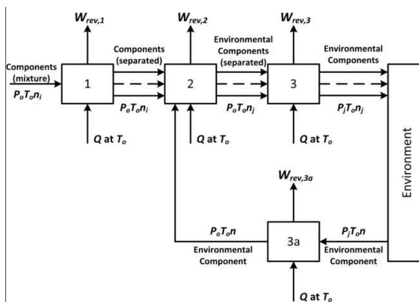
Figure 4. Scheme for Calculating Chemical Exergy of Mixtures
