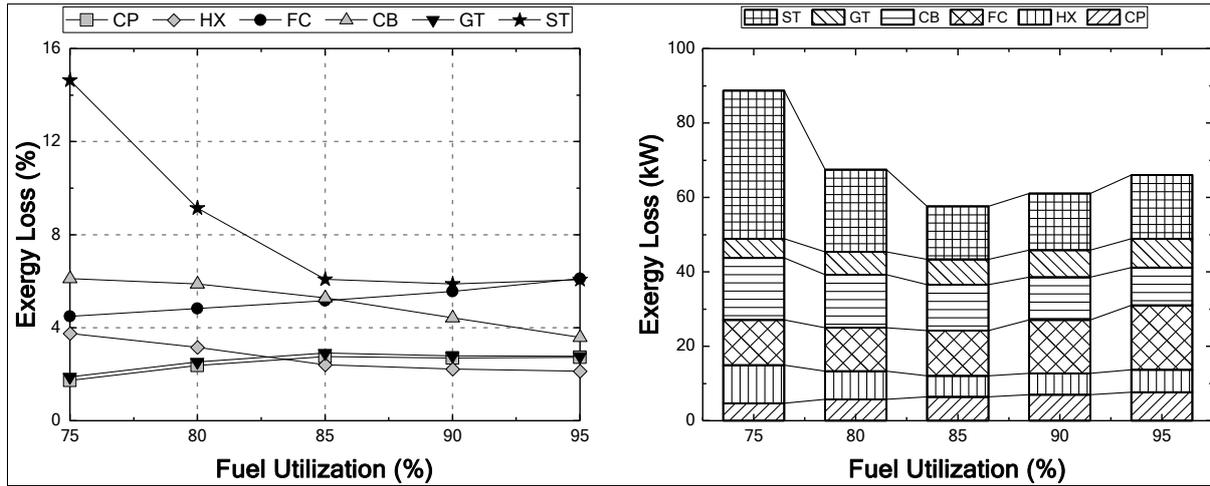
Figure 22. Exergy Loss variation v/s Fuel Utilization - Methane
