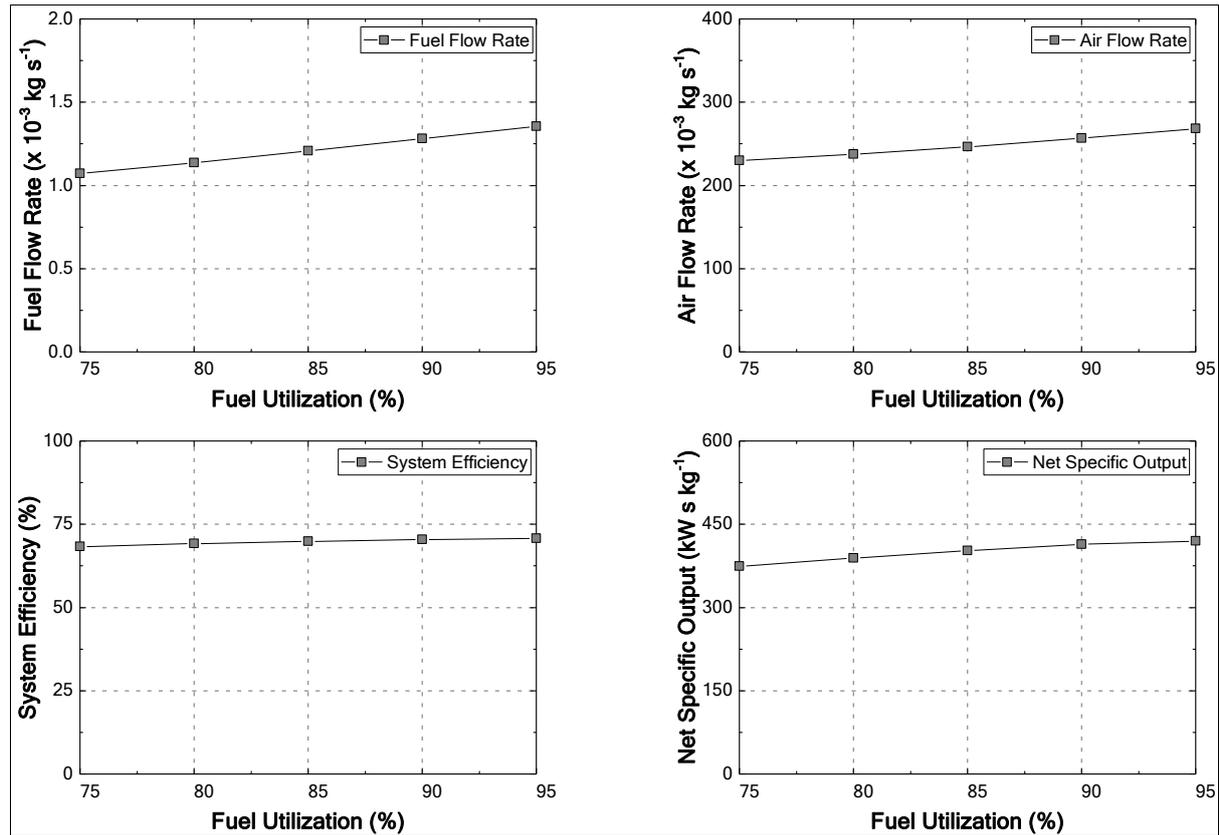
Figure 15. Trends in System Variables v/s Fuel Utilization - Hydrogen
