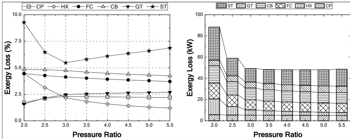
Figure 19. Exergy Loss variation v/s Pressure Ratio - Methane
