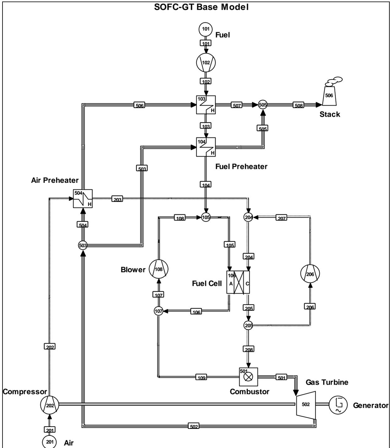
Figure 6. Base case system model in Cycle Tempo
