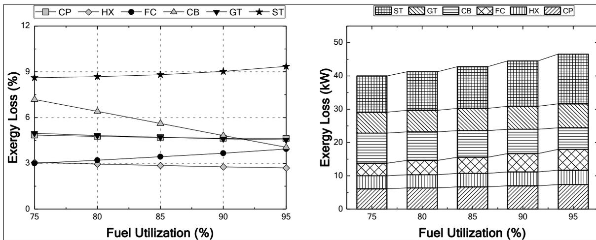
Figure 14. Exergy Loss variation v/s Fuel Utilization - Hydrogen
