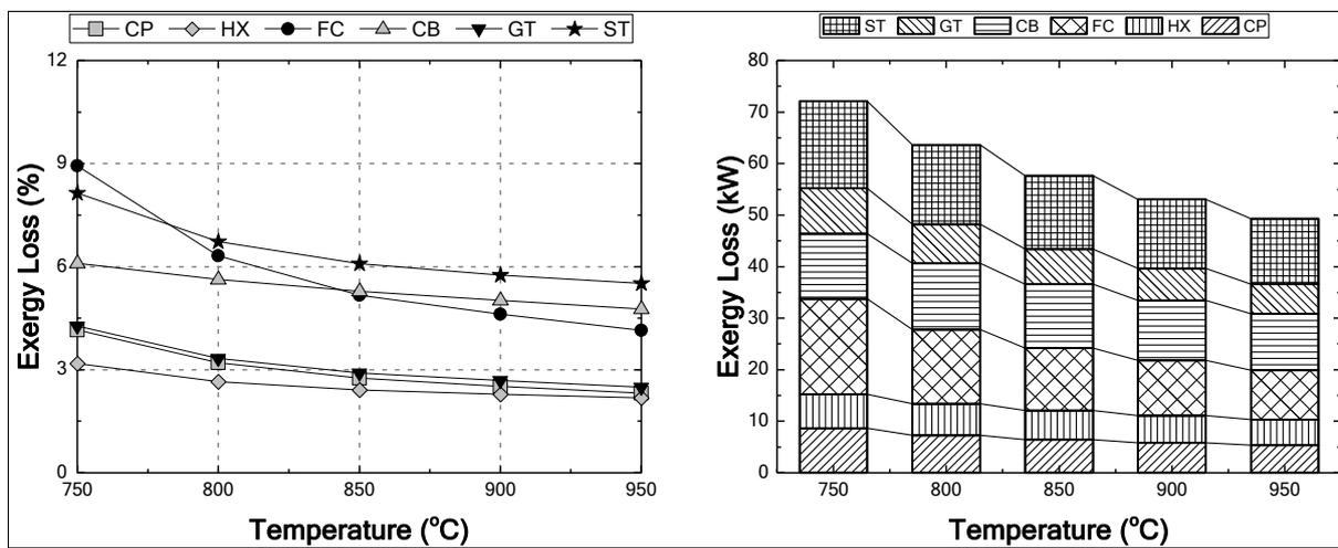
Figure 17. Exergy Loss variation v/s Cell Temperature - Methane
