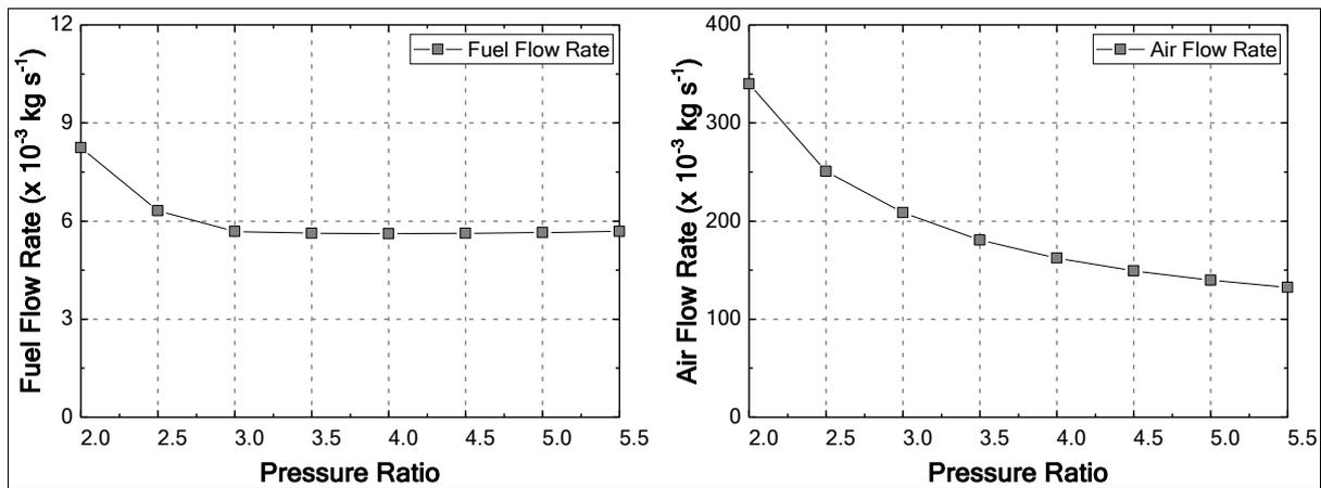
**Figure 18.** Fuel Flow, Air Flow v/s Pressure Ratio – Methane
