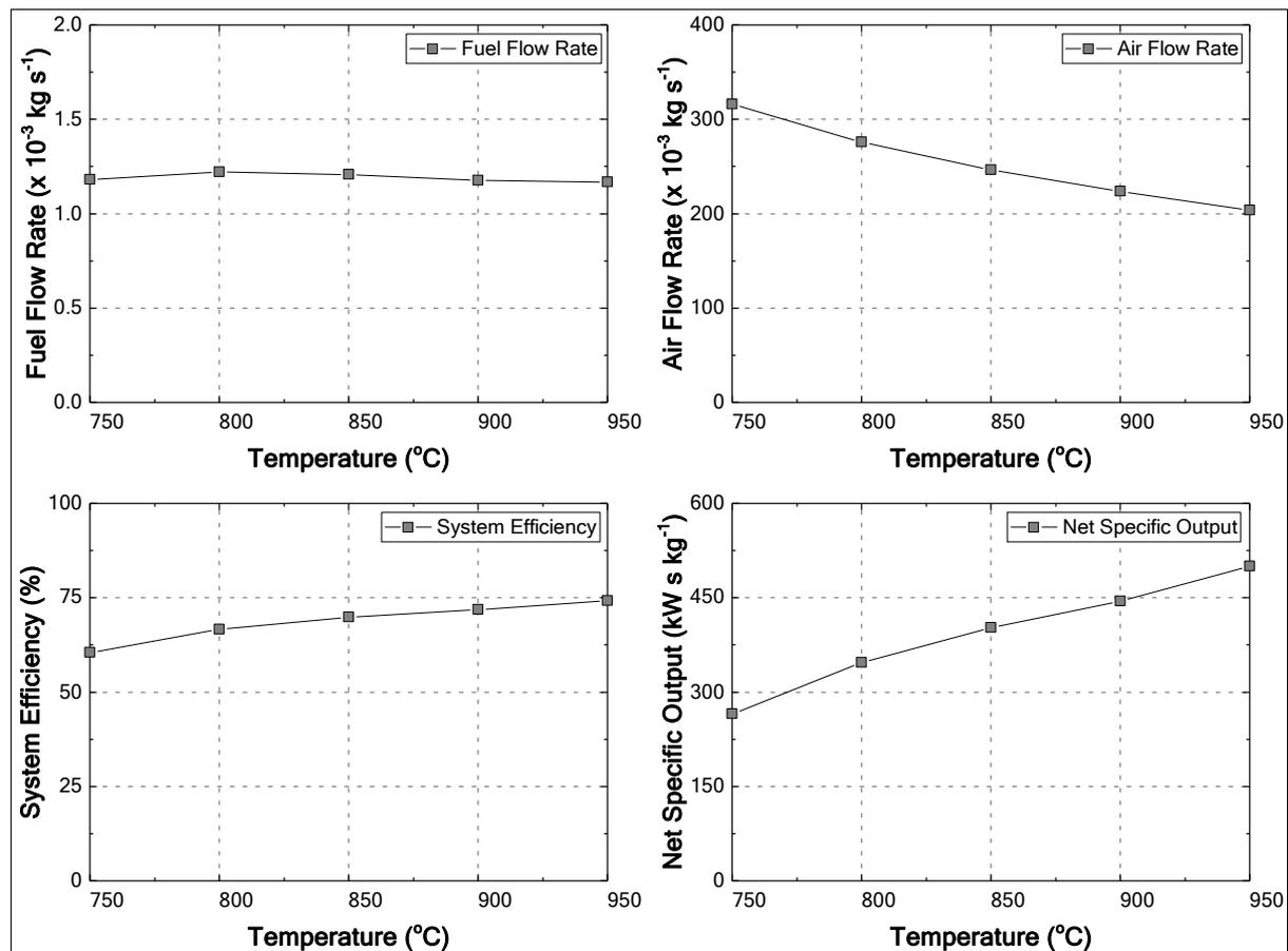
Figure 10. Trends in System Variables v/s Cell Temperature - Hydrogen
