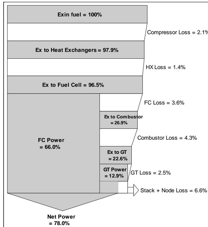
Figure 27. Exergy flow diagram – Methane Optimized
