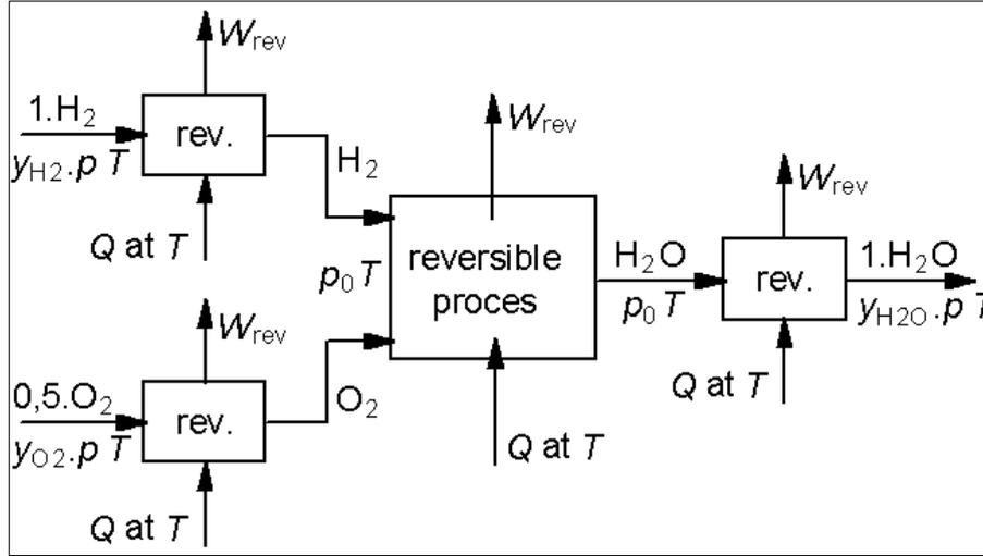
**Figure 2.** Thermodynamic model of a reversible ( $\text{H}_2\text{-O}_2$ ) isothermal fuel cell
