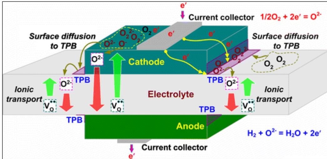
Figure 1. Schematic of an SOFC showing relevant transport processes [44]
