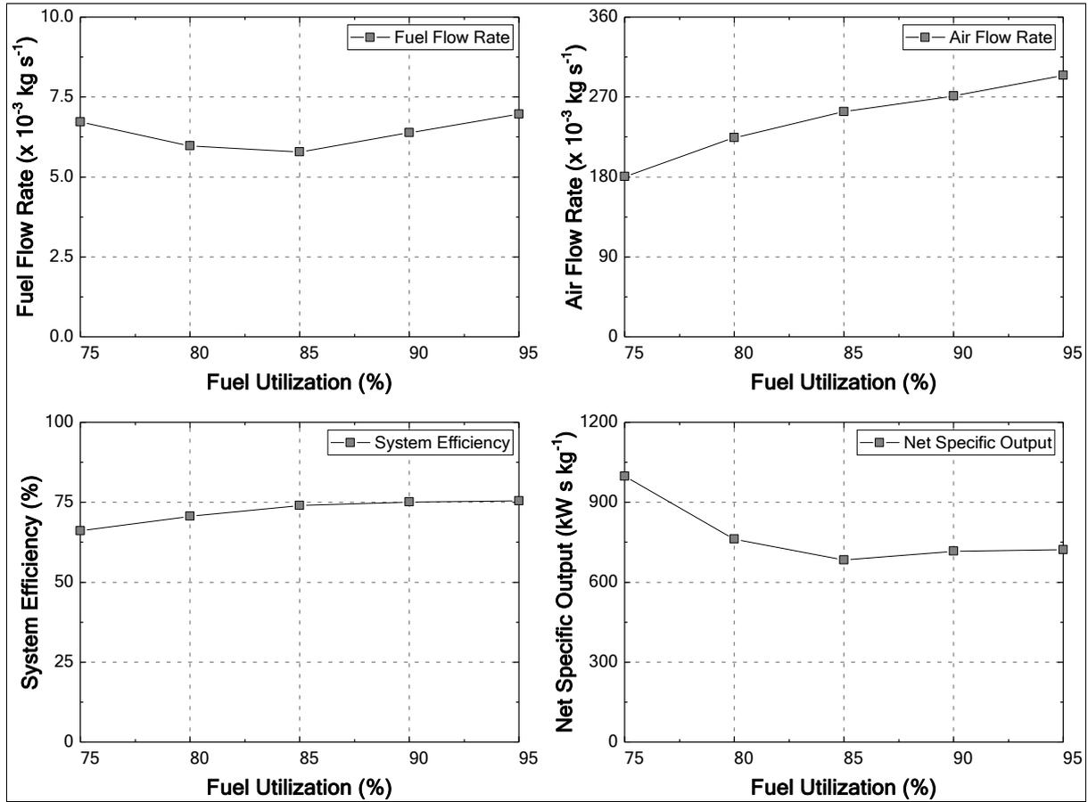
Figure 21. Trends in System Variables v/s Fuel Utilization – Methane
