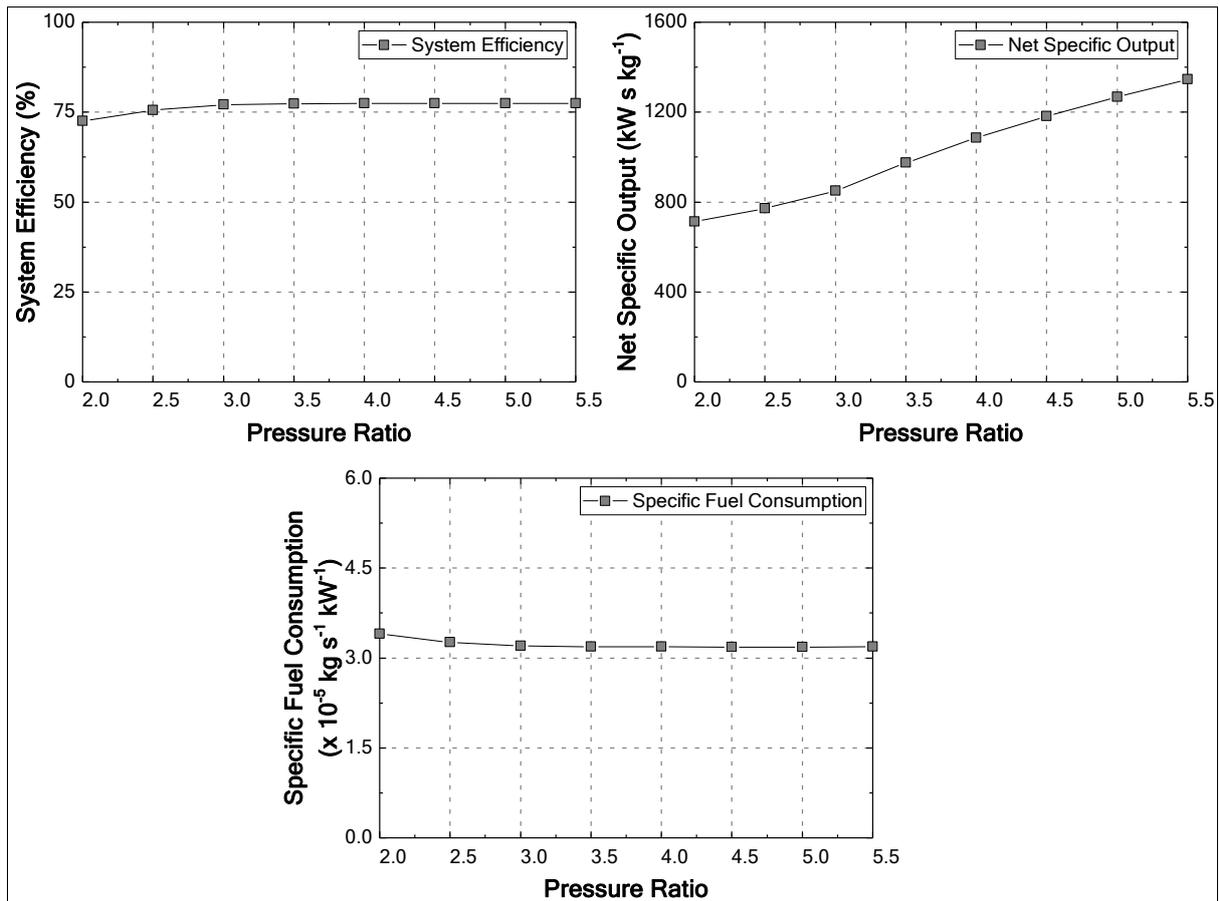
Figure 20. System Efficiency, Net Specific Output, Specific Fuel Consumption v/s Pressure Ratio – Methane
