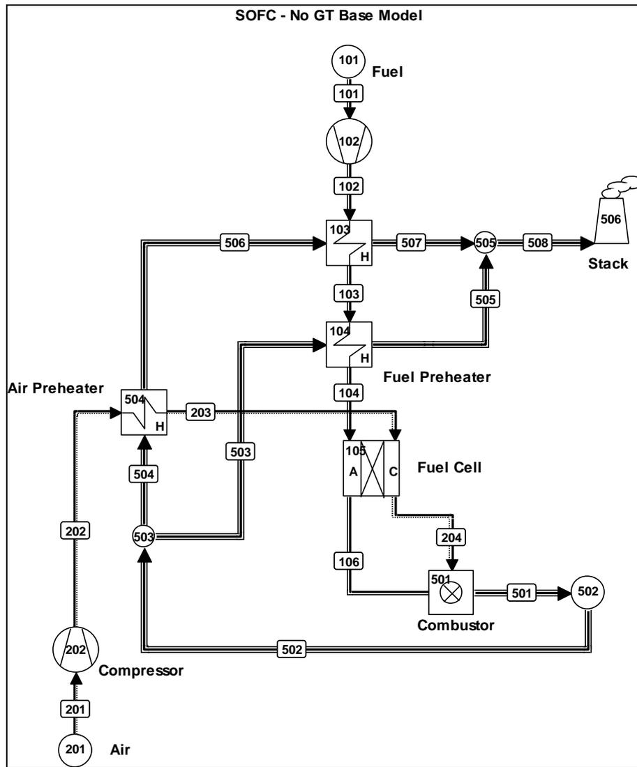
Figure 28. Base model without Gas Turbine
