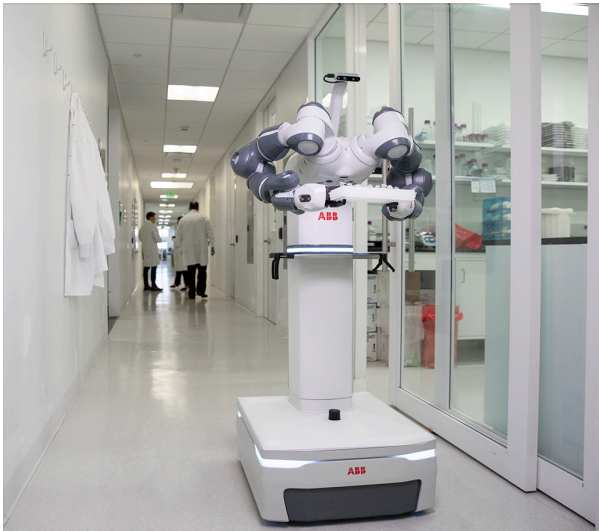
(a) ABB's mobile and autonomous YuMi laboratory robot concept designed to work alongside medical staff and lab workers [15]
