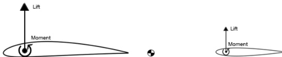
Figure 6.1: Longitudinal stability of a conventional aircraft
