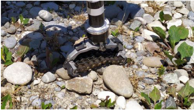
FIGURE 3. The SoftFoot-Q [87], a compliant foot designed to be robust and to adapt to the terrain.
