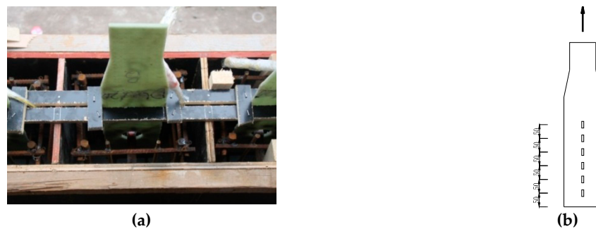
Figure 3. Specimen's fabrication. (a): Fabrication process; (b) Strain gauges on SC-P, (unit: mm).
