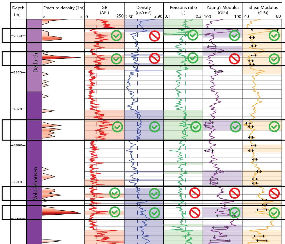
Figure 6.5: Distribution of fractures on the VAL-01 image log compared to the mechanical properties. The high fracture density within the black box, highlighted density above 2.65 gr/m 3 (blue), the Poisson's ratio above 0.21 (green), Young's (purple), Shear modulus fluctuation (yellow). The arrow indicate fluctuation over the minimum fluctuation of 30 GPa/m and 20 GPa/m for Young's and Shear modulus respectively and the 150 API/m fluctuation for the gamma ray log. A positive correlation is indicated by a green check-mark and a negative correlation by a red cross
