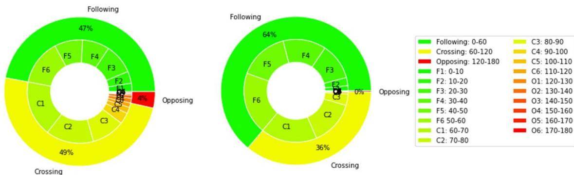
Figure 40: Probability of direction of wave trains compared to the most energetic wave train for multimodal wave spectrums, with a threshold of 0.5 m left and 1 m right, containing 75% and 37% of the data, the layout of the graph and considered location is similar to that of Figure 36.
