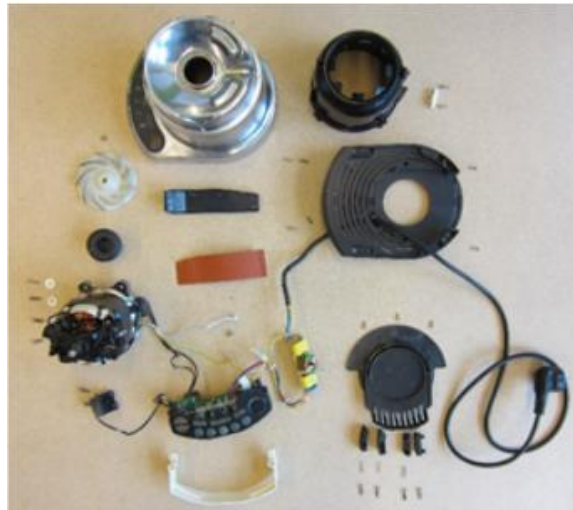
Figure 4. Disassembled motor assembly of the Solis Household blender
