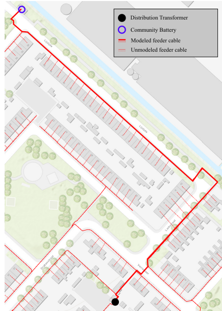
Figure 4.7: GIS view of Alliander's low voltage network of Rijsenhout. The outlined modeled network is the network that is considered for the DGSE model. The modeled part of the network consists of 34 customers. The unmodeled cables are not physically connected to the modeled network. At the distribution transformer and the community battery both power and voltage are measured. At 12 households, the power was measured. For privacy reasons, their exact location could not be displayed, but they are almost uniformly distributed along the cable.
