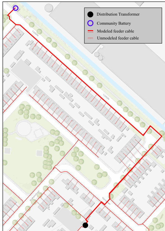
Figure 2.4: GIS view of Liander's low voltage network of Rijsenhout. [27] The outlined modeled network is the feeder that is considered for the LV model. The unmodeled cables are not physically connected to the modeled network, except for a connection in de MV/LV transformer.
