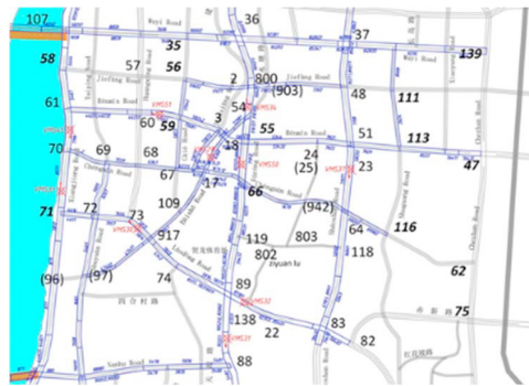
Figure 1 The road network of the CBD of Changsha. The intersections with bold numbers have ANPR
