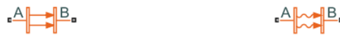
Figure 4.5: Simscape "components" that calculate radiative- (left) and convective- heat flow between defined cell elements.
