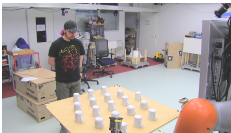
Figure 3: Experimental setup for evaluating readability of avatar gaze targets. The participant stands 2m from the screen at varying angles. Adjacent cups on the table are 20cm from center to center. All cups are 7.5cm in diameter.
