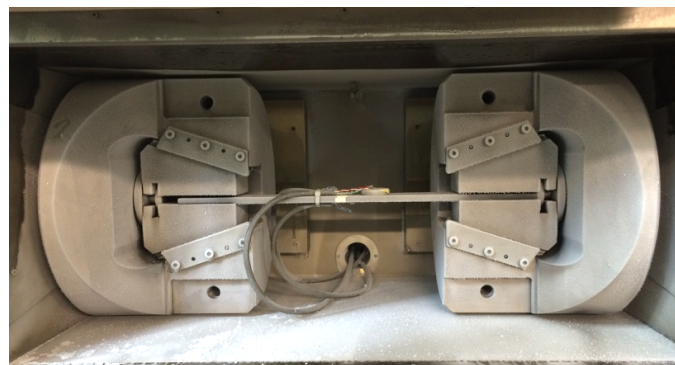
Fig. 3. Fatigue testing climate chamber at TUHH.
