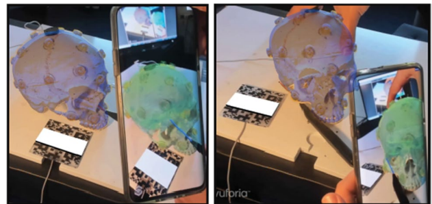
Fig. 15 Augmented images of the phantom skull and the pointer. The pictures show a collaborative augmented reality scenario where the blue skull is the desktop's view and the green skull is from the smartphone point of view. The left image showcases the instrument augmentation in both devices, while the right one represents the projections after moving the multimodal marker and the skull
