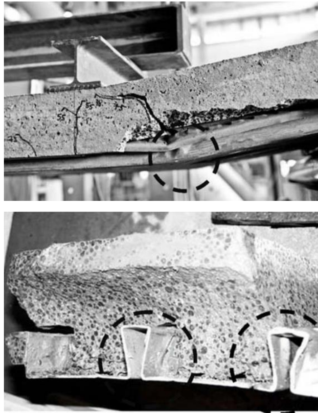
Figure 2.30 – Buckling of the webs at the location of the inclined crack[27]
