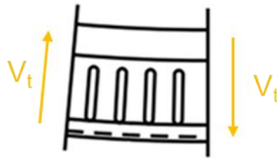
Figure 1.8 – Transverse shear force[23]
