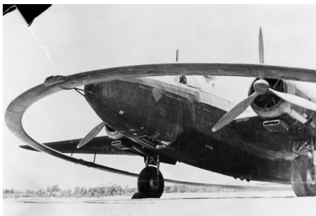
Figure 1.1: Wellington bomber with coil to set off magnetic mines.
