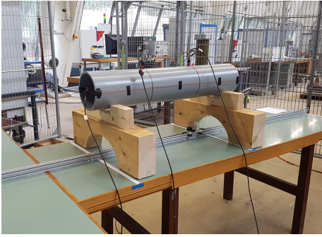
Figure 2.4: Metal pipe with three copper degaussing coils; one in the M and two in the L-direction.
