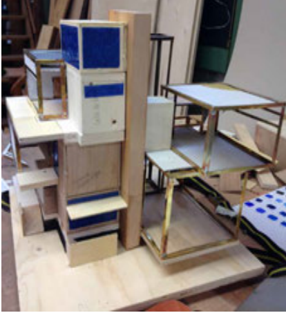
FIG. 29 The differences in height between the different building elements, equalised with wooden boards of different thicknesses, 20 April 2017. Photo Nico Bodewes
