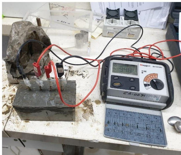
Figure 3: The Megger wenner probe consists of a resistance meter, four electrodes and an EC box
