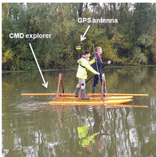
Figure 2: The CMD explorer is made waterborne by a surfboard construction for this study
