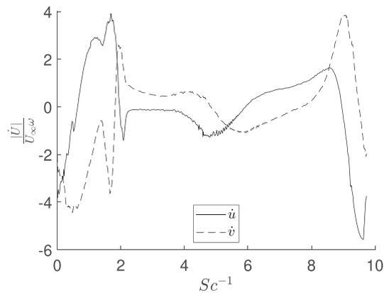
**FIGURE 9** Acceleration vs. distance over boundary surface
