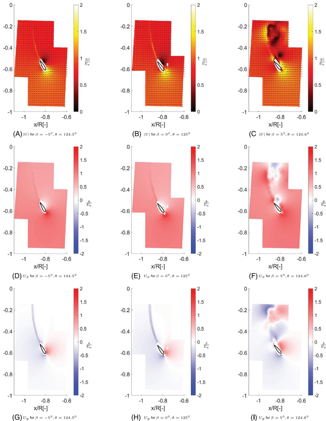
**FIGURE 20** Quiver and color plot of the velocity magnitude, velocity in x direction, and velocity in y direction for  $\theta = 120^\circ$  position [Colour figure can be viewed at [wileyonlinelibrary.com](http://wileyonlinelibrary.com)]
