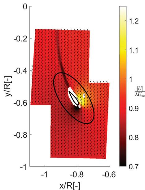
**FIGURE 24** Velocity field in the airfoil reference frame at the 120° position [Colour figure can be viewed at [wileyonlinelibrary.com](https://onlinelibrary.wiley.com)]
