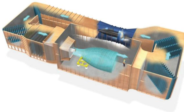
**FIGURE 4** Schematic of Open Jet Facility at TU Delft [Colour figure can be viewed at [wileyonlinelibrary.com](https://onlinelibrary.wiley.com)]
