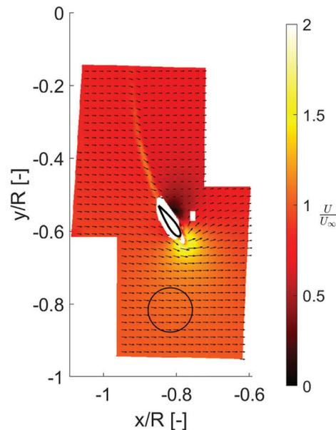
**FIGURE 11** Velocity magnitude at  $\theta = 125^\circ$  with a test boundary surface not encompassing the airfoil.  $F_n = 1.8e - 3$ ,  $F_t = 3.48e - 4$  [Colour figure can be viewed at [wileyonlinelibrary.com](http://wileyonlinelibrary.com)]
