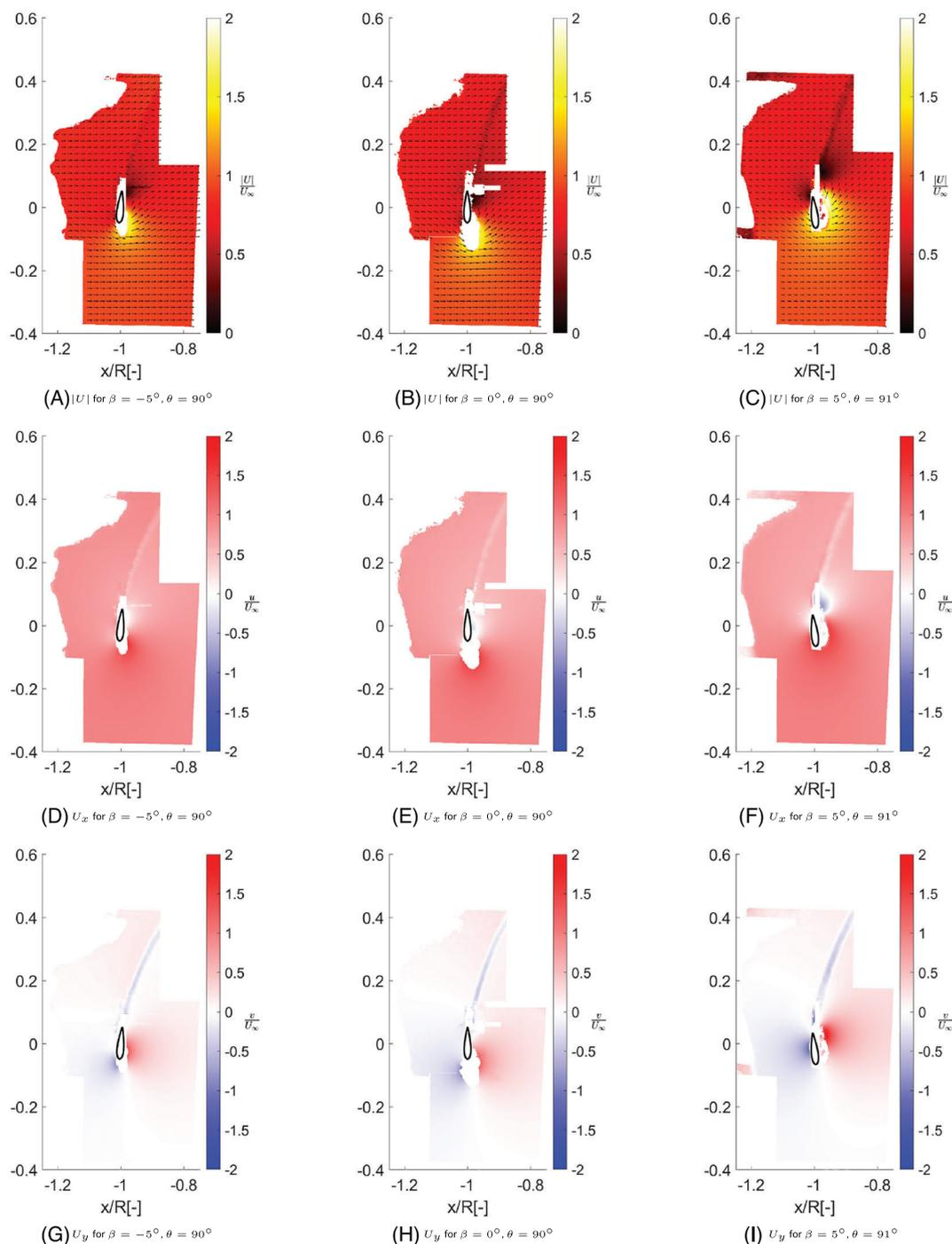
**FIGURE 19** Quiver and color plot of the velocity magnitude, velocity in x direction, and velocity in y direction for  $\theta = 90^\circ$  position [Colour figure can be viewed at [wileyonlinelibrary.com](http://wileyonlinelibrary.com)]
