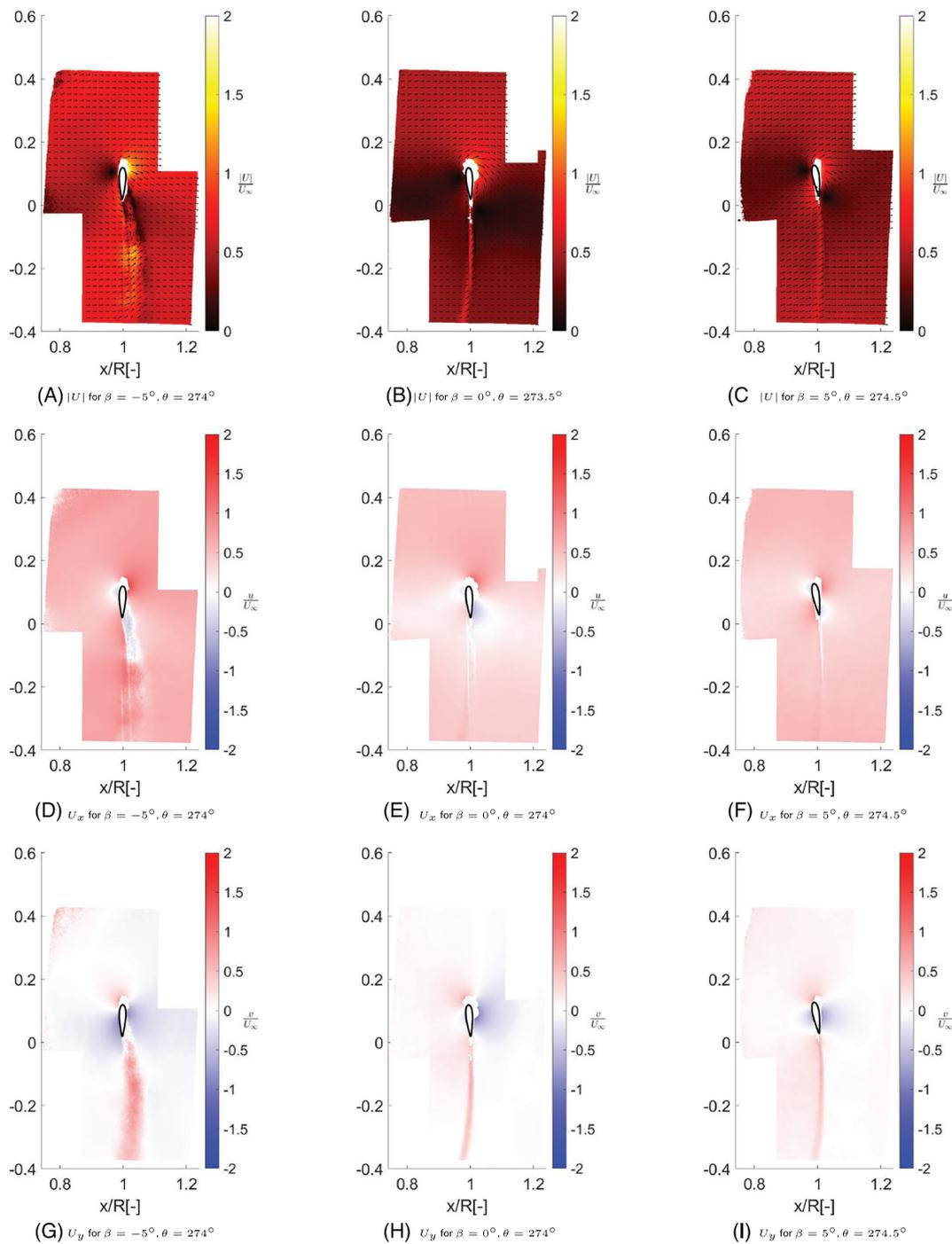
**FIGURE 21** Quiver and color plot of the velocity magnitude, velocity in x direction, and velocity in y direction for  $\theta = 270^\circ$  position [Colour figure can be viewed at [wileyonlinelibrary.com](http://wileyonlinelibrary.com)]
