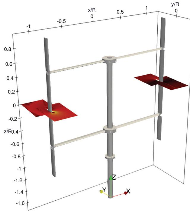
**FIGURE 6** PitchVAWT turbine showing the measurement planes at locations  $\theta = 90$  and  $\theta = 270$  [Colour figure can be viewed at [wileyonlinelibrary.com](http://wileyonlinelibrary.com)]
