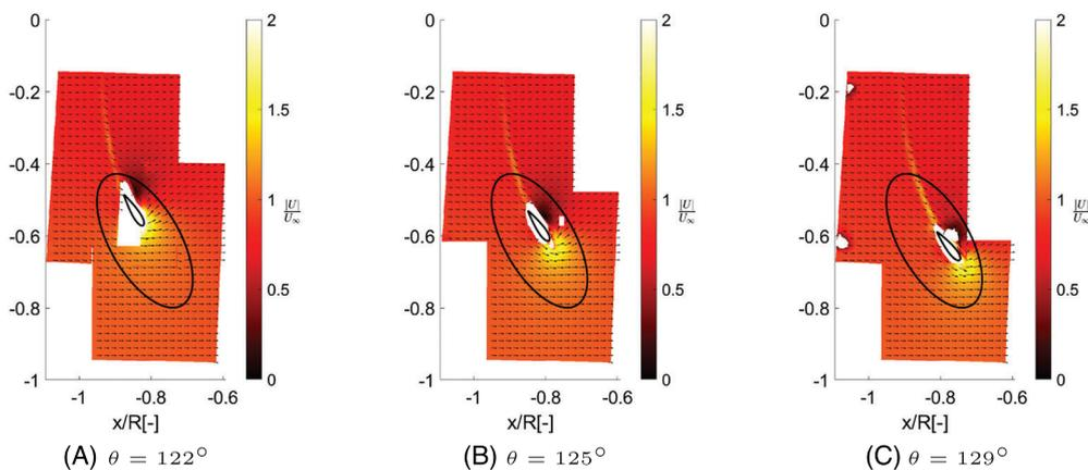
**FIGURE 7** Velocity magnitude of each measurement section; the boundary surface shown as the blue oval envelopes each azimuthal position [Colour figure can be viewed at [wileyonlinelibrary.com](http://wileyonlinelibrary.com)]
