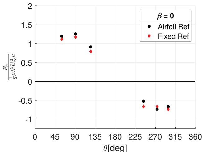
**FIGURE 25** Comparison of normal load calculation in fixed and rotating reference frames [Colour figure can be viewed at [wileyonlinelibrary.com](https://onlinelibrary.wiley.com)]
