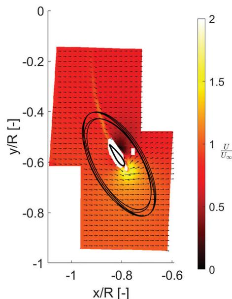
**FIGURE 12** Various surface boundaries encompassing the airfoil positions. Results given in Table 3 [Colour figure can be viewed at [wileyonlinelibrary.com](http://wileyonlinelibrary.com)]
