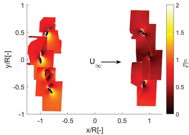
**FIGURE 15** Velocity magnitude with a  $\lambda = 4$  and  $\beta = 5$  [Colour figure can be viewed at [wileyonlinelibrary.com](http://wileyonlinelibrary.com)]
