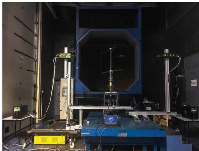
**FIGURE 5** PitchVAWT mounted in the Open Jet Facility with opposing synchronized PIV lasers, cameras, and traversing system [Colour figure can be viewed at [wileyonlinelibrary.com](https://onlinelibrary.wiley.com)]
