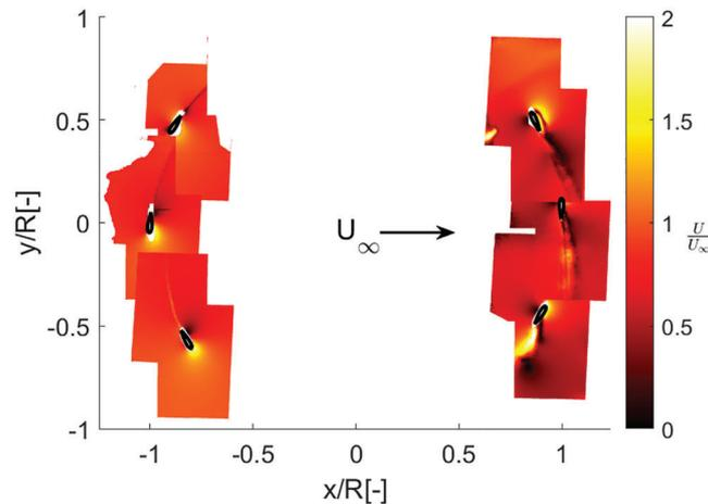
**FIGURE 17** Velocity magnitude with a  $\lambda = 4$  and  $\beta = -5$  [Colour figure can be viewed at [wileyonlinelibrary.com](http://wileyonlinelibrary.com)]
