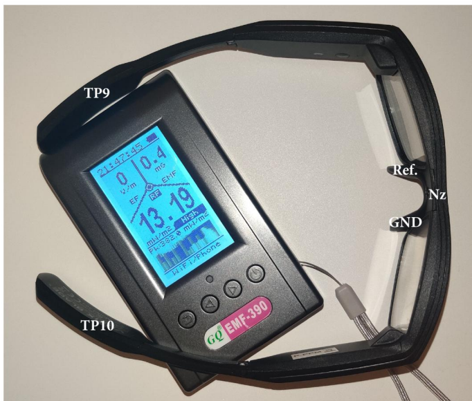
(a) Only the TP9 electrode location displayed high RFF periodically (max. 382 \text{ mW}/\text{m}^2 ) hinting at an internal Wi-Fi antenna as indicated by the GQ EMF-390 meter.
