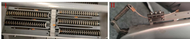
Fig. 20. Visualizations of spring configuration for thigh joint (left column) and the PEA for the calf joint (right column).
