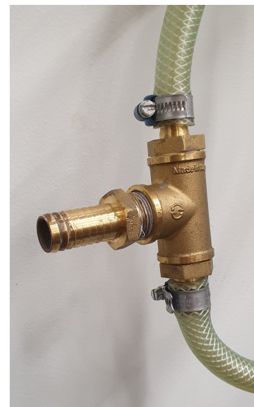
Figure 2.5: Picture of a brass hose tail and the flexible PVC hoses.
