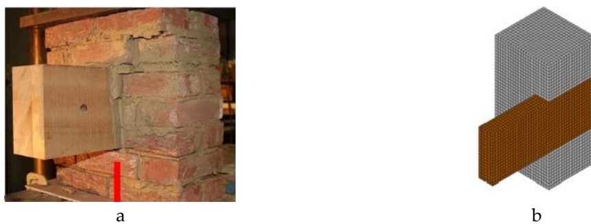
Figure 2.36: Mud mortar masonry and timber – (a) Pull-out test, and (b) Numerical model from [89]
