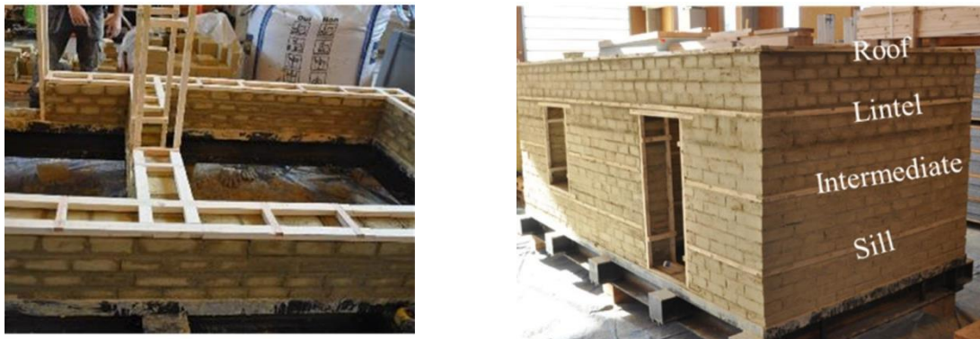
Figure 2.27: Shake table testing for timber-reinforced earth block masonry [73]
