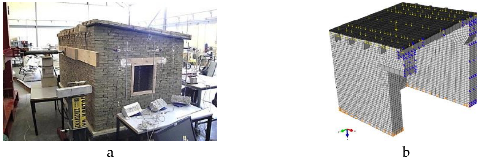
Figure 2.40: 1:2 scale adobe masonry building – (a) Physical model, and (b) Numerical model from [95]
