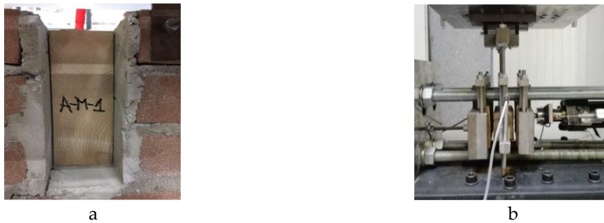
Figure 2.35: a) Timber joist and brick masonry, frictional behaviour from [87], and b) Cyclic friction triplet test setup between mortar and timber from [88]
