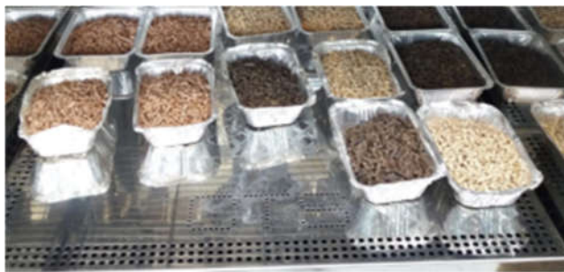
Figure 1. Pellets on aluminum trays in the climate chamber. This figure is an example showing the pellets on aluminum trays. The same trays were used for the other storage conditions.
