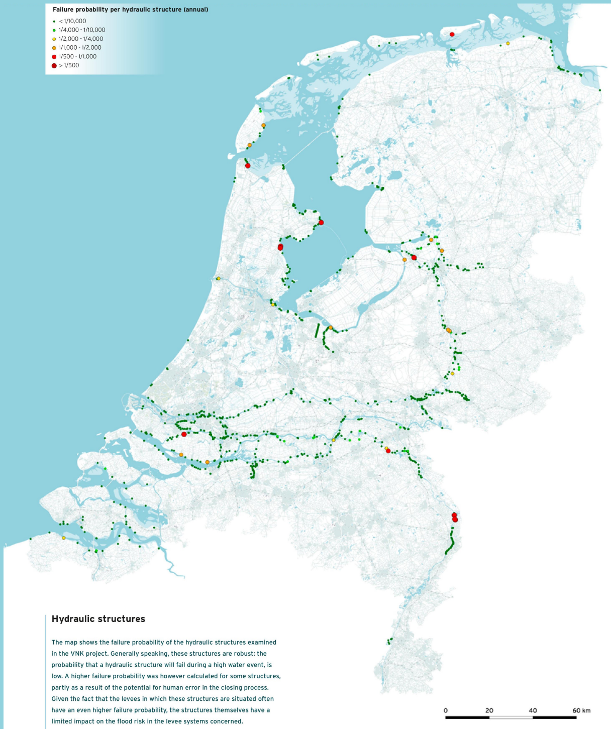
Figure 6.5: The Failure Probability of Hydraulic Structures in the Netherlands (VNK Project Office, 2016)
