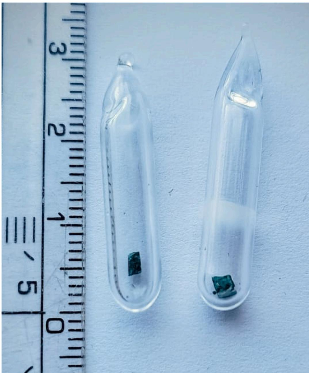
Fig. 1. Millimeter sized crystals of NaI:0.2%Sm<sup>2+</sup> (left) and NaI:0.2%Tl<sup>+</sup>,0.2%Sm<sup>2+</sup> (right) crystals sealed in silica ampoules.
