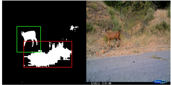
Figure 3: A segmentation where the deer is segmented out, but also another larger part of the image is segmented, causing the IoU score to be lower.
