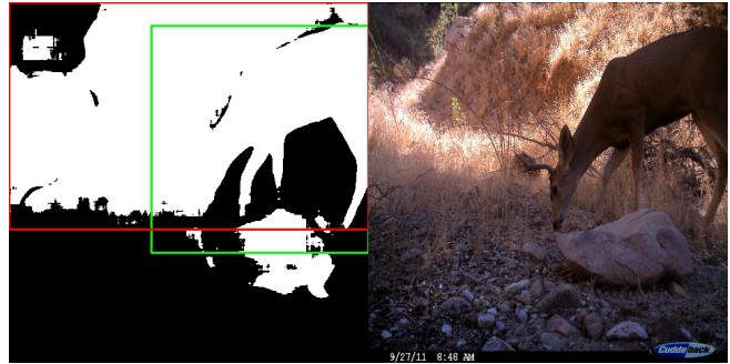
Figure 5: An overexposed segmentation where the background is segmented as well and this part is connected to the segmentation of the deer.
