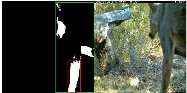
Figure 4: A separated segmentation of a deer, which causes the IoU score to be lower because only the largest segmentation is compared to the ground truth.
