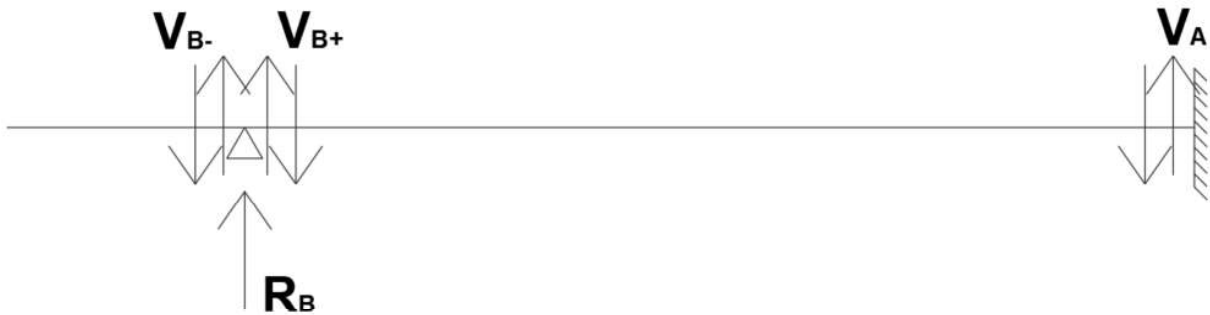
Figure 11.5, Definition of shear and reaction forces.
