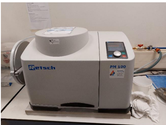
Figure 3.1: Retsch Planetary Ball Mill PM 100
