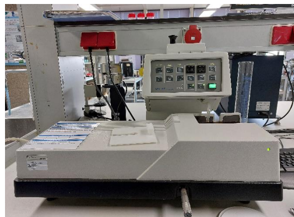
Figure 3.2: EyeTech Particle size and shape analyzer
