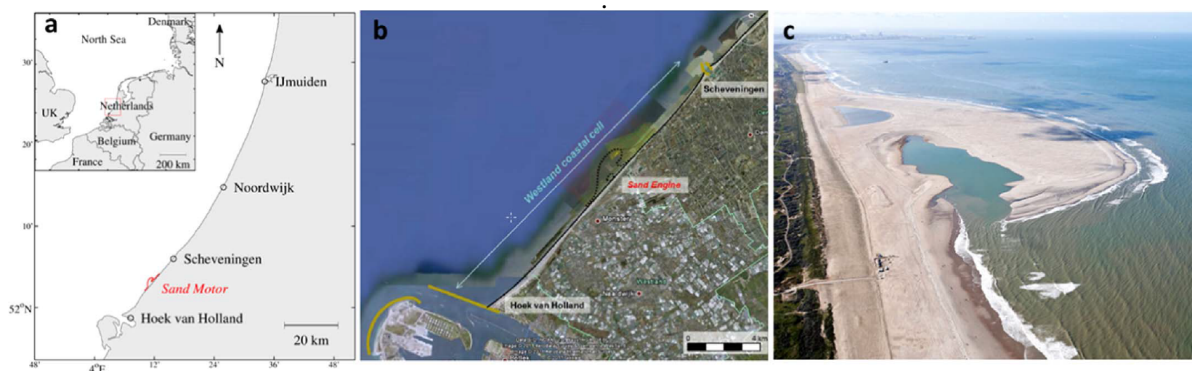
Figure 3.1: a) Location of the Sand Engine along the Holland Coast. b) The Westland coast. c) aerial photograph of the Sand engine in July 2011 after construction (courtesy: Rijkswaterstaat/Joop van Houdt). After Luijendijk et al. (2017)
