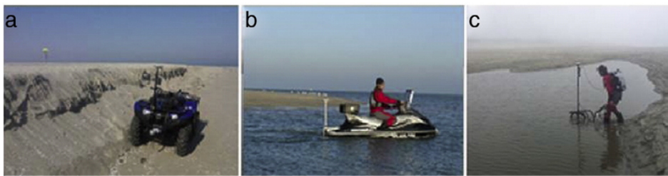
Figure 3.6: Survey techniques. a) 4WD quad, b) jetski, c) wheeled pole. From De Schipper et al. (2016).
