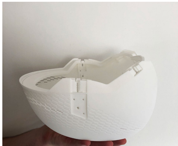
Fig. 92 — Hardshell-Access prototype setup Testing the assembly of hardshell towards Base-Ring.
