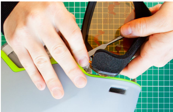
Fig. 45 – Visor-removal with help of a metal spudger
