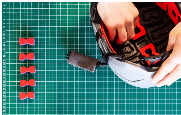
Fig. 34 — Remove inside parts
