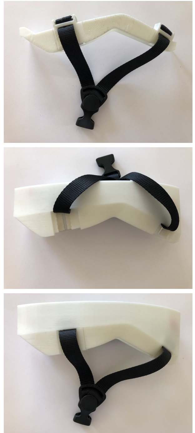
Fig. 96 — Chinstrap as fixation element (functional test)
