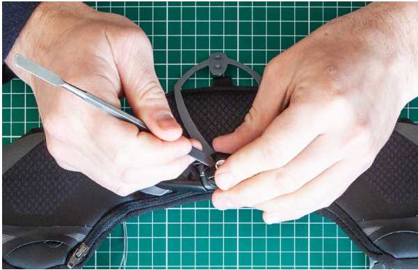
Fig. 43 – Using a metal spudger to remove BOA-pin
