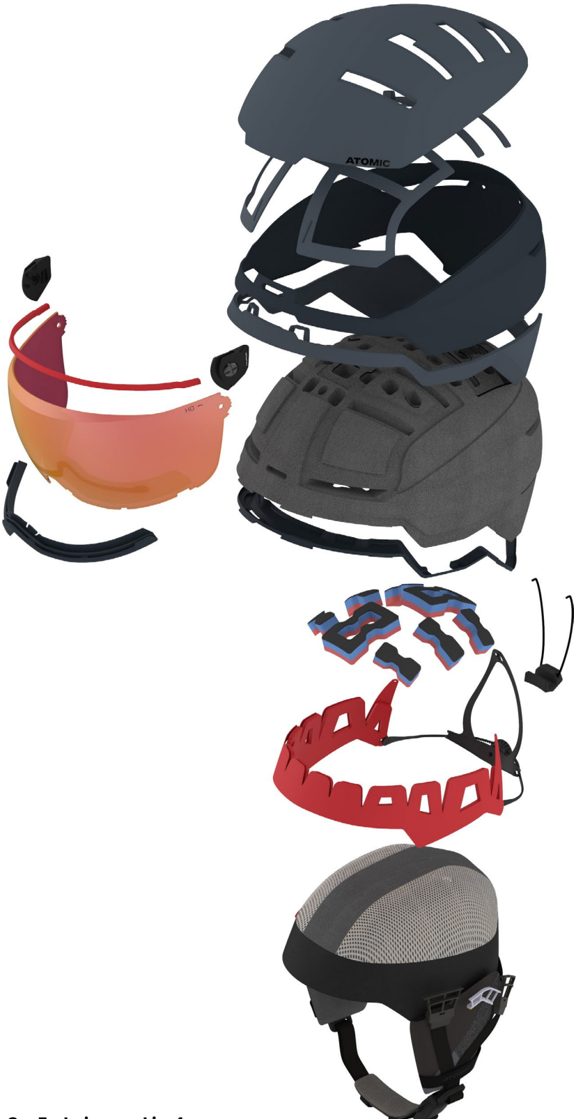
Fig. 3 – Explosion graphic of current Atomic helmets
