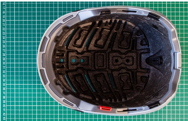
Fig. 53 — Remaining in-mold assembly parts
