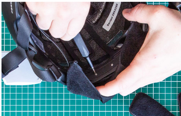
Fig. 50 – Removing the POC fitting-system
