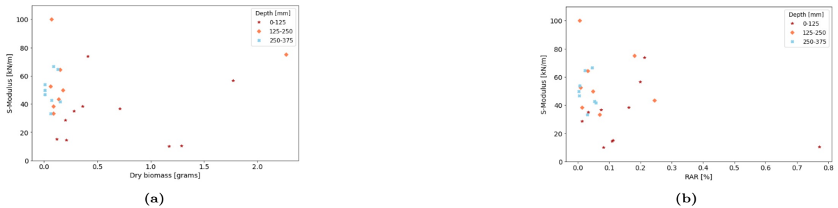
Figure 4.23: Corkscrew extraction test results at each depth levels for individual soil samples containing roots of S. fragilis . The S-modulus versus (a) the root biomass and (b) the root area ratio.
