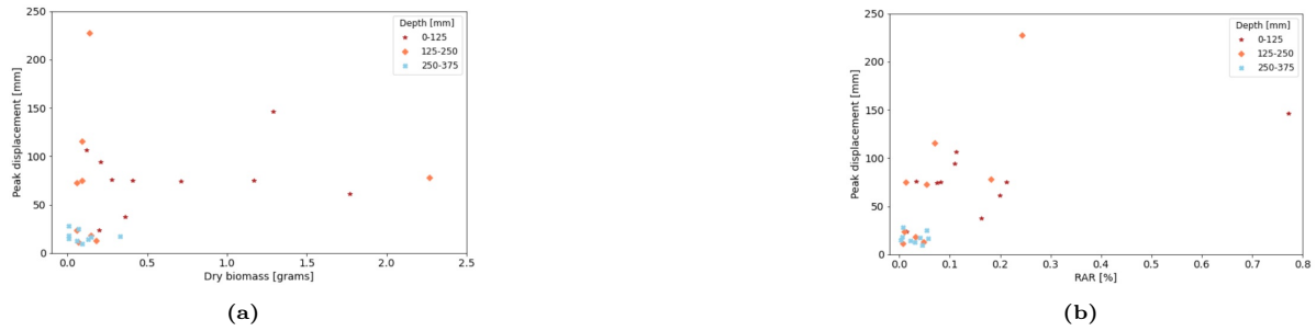
Figure 4.25: Corkscrew extraction test results at each depth levels for individual soil samples containing roots of S. fragilis . The peak displacement versus (a) the root biomass and (b) the root area ratio.
