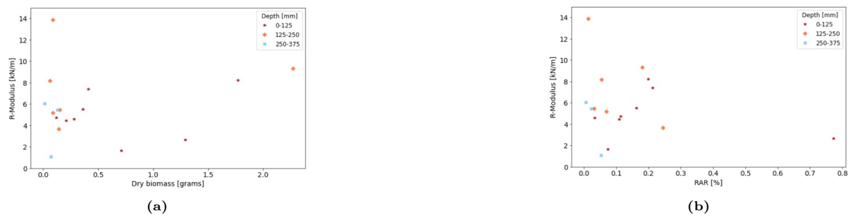
Figure 4.24: Corkscrew extraction test results at each depth levels for individual soil samples containing roots of S. fragilis . The R-modulus versus (a) the root biomass and (b) the root area ratio.
