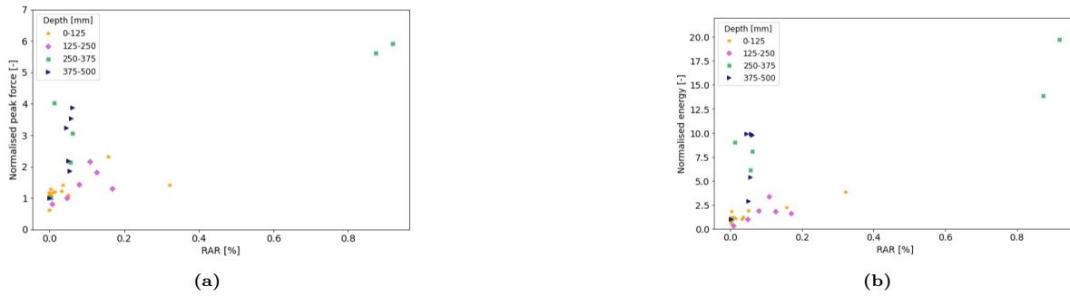
Figure 4.31: Corkscrew extraction test results at each depth levels for individual soil samples containing roots of S. purpurea . (a) The normalised peak force versus the root area ratio and (b) the normalised energy versus the root area ratio.
