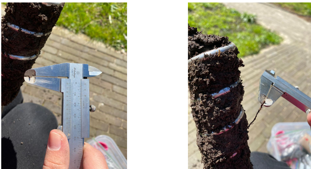
Figure 3.10: Determination of the diameter of the broken roots with a Vernier caliper.
