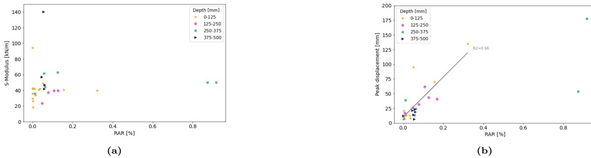
Figure 4.32: Corkscrew extraction test results at each depth levels for individual soil samples containing roots of S. purpurea . (a) The S-modulus versus the root area ratio and (b) the peak displacement versus the root area ratio, a fitted line was drawn for all depth levels combined.
