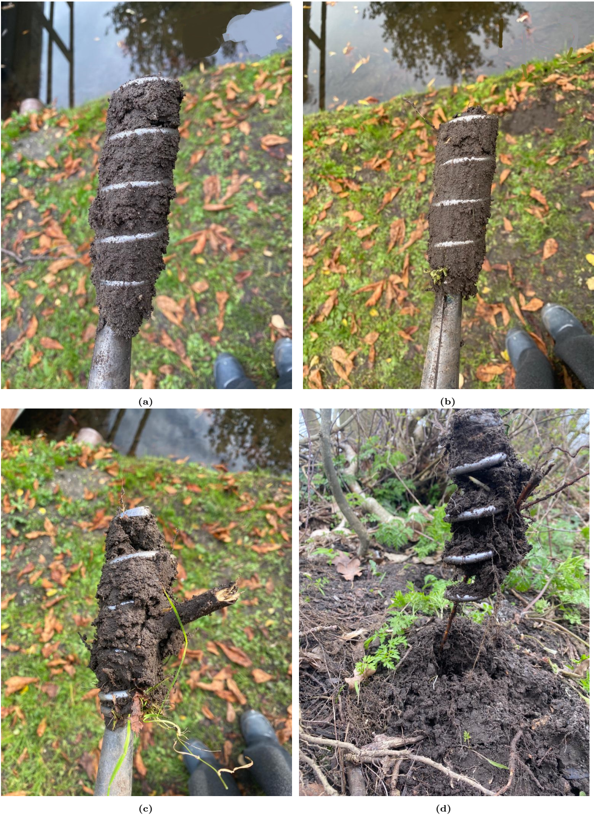
Figure 3.11: Example of the different types of samples (a) with no roots, (b) with thin roots, (c) with a thick root and (d) with a slipped root.
