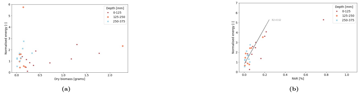
Figure 4.22: Corkscrew extraction test results at each depth levels for individual soil samples containing roots of S. fragilis . The corkscrew normalised peak energy versus (a) the root biomass and (b) the root area ratio, a fitted line was drawn for all depth levels combined.
