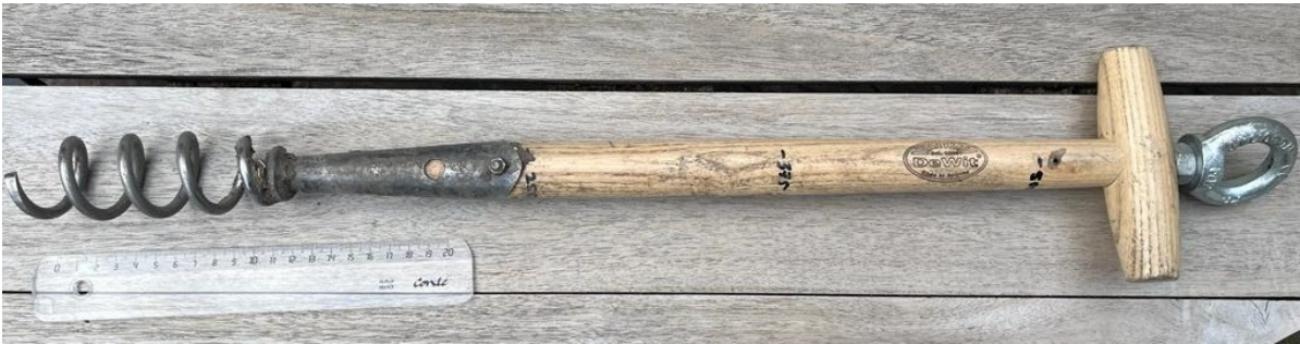
Figure 3.4: Picture of the corkscrew weeder (De Wit, Kornhorn, The Netherlands); height h_{cs} = 125 mm, diameter d_{cs} = 40 mm
