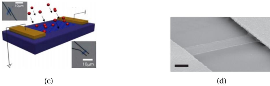
Figure 1.2: (a) Suspended graphene resonator [16] (b) Graphene pressure sensor [21] (c) Graphene based NO<sub>2</sub> gas sensor [22] (d) SEM image of suspended graphene resonator with electrical contacts [18]
