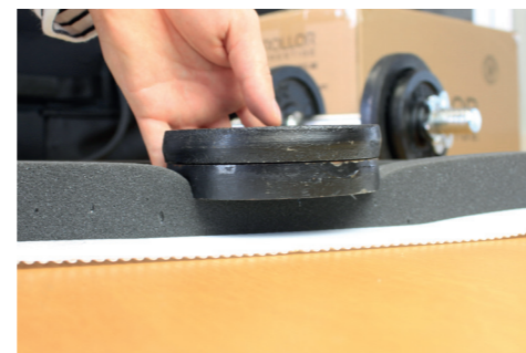
Figure 6 Result of the T33260 foam being compressed for four weeks. Full result of test can be found in Chapter Roll up test.
