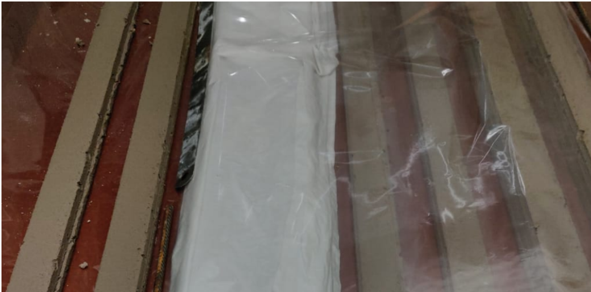
(a) Samples without curing on the left, samples covered with a wet burlap in the middle, and samples covered with a plastic film on the right.
