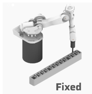
(b) Robotic-arm printer (CyBe)
