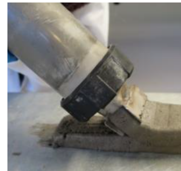
(c) Hybrid-flow, rectangular extrusion (Rubio et al., 2017).
