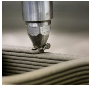
(a) Down flow, circular extrusion (3Dnatives).
