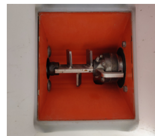
(c) Screw extrusion mechanism
