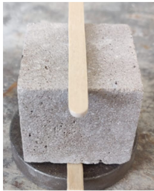
(c) Sample for the tensile splitting test
