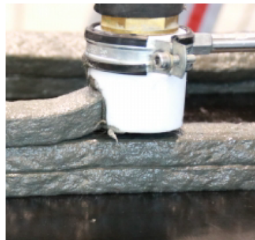
(b) Back-flow, rectangular extrusion (Ogura et al., 2018).
