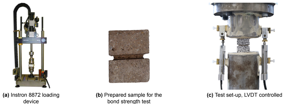
Figure 3.2: Reference, sample, and test set-up for the bond strength test.
