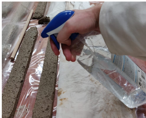
(b) Samples sprayed with water, every 30 minutes or 1 hour.
