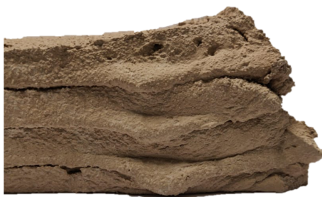
(c) Excess of material at beam end - side view
