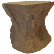
Figure 3.23: Impression of the failure mechanism that was observed the most. The filaments are positioned horizontally, but not visible in this figure.
