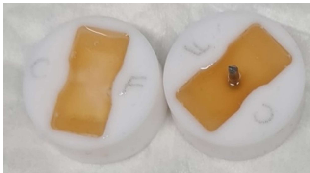
Figure 2.1: The mold used to prepare the PRP tensile test sample is shown on the left. On the right, the same mold includes a rod in the middle to ensure a 2 mm hole necessary for the fracture test samples. The shape and size of the molds used for the tensile and fracture test are identical.
