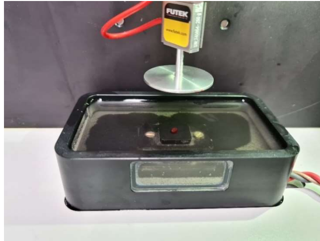
Figure 2.4: Compression test set-up. The clot analog is placed in the 37 °C degrees DMEM bath. 80% compression for 20 cycles will be performed on the clot analog.
