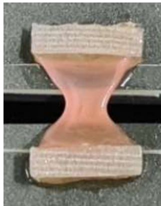
Figure 2.3: Placement of the sample on the clamps of the tensile tester. Visible are the sandpaper, double-sided foam tape, and Velcro taps.
