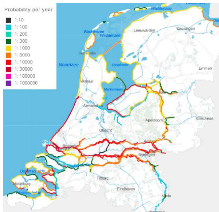
Figure 2.3: Location of the primary dike segments according to the new safety standards of 2017. Obtained from the website Waterveiligheidsportaal (“Waterveiligheidsportaal”, 2020).
