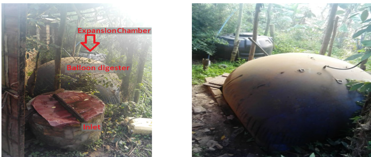
Figure 7. Balloon type digester.
