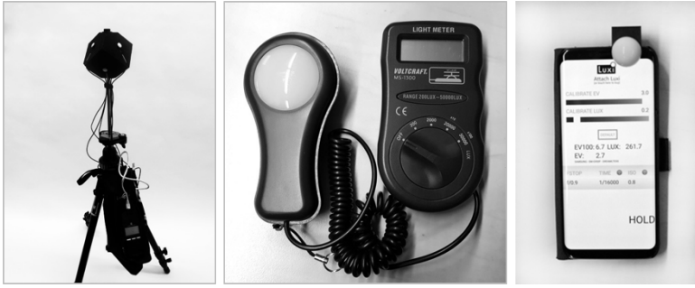
Figure 6.13: Measurement devices. Left to right: cubic meter based on Konica Minolta system (Xia et al., 2016ab), luxmeter, smartphone with Luxi.
